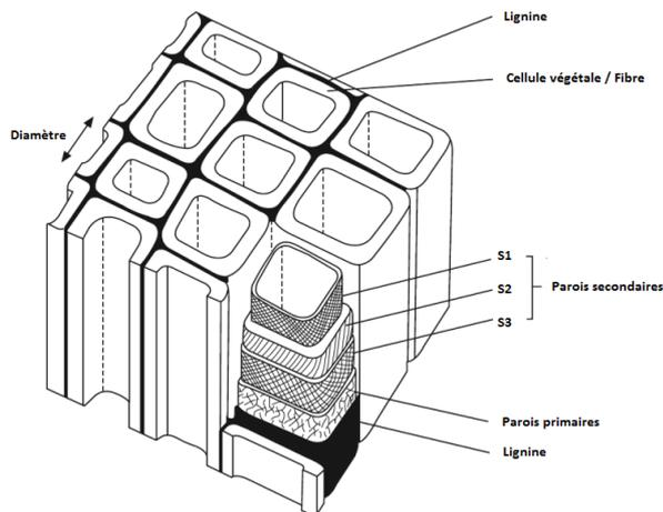
**Figure 3:** Structure of vegetal cellulosic fibers.
